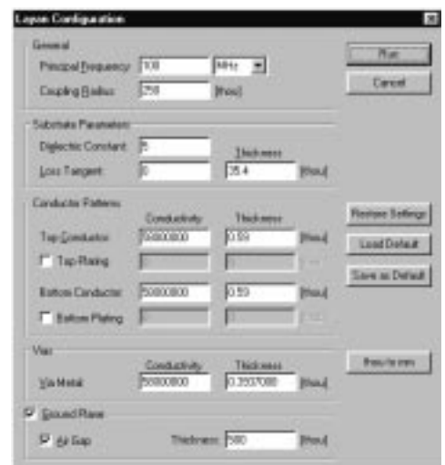
Physical PCB parameters for Layan are set-up using one dialog!
